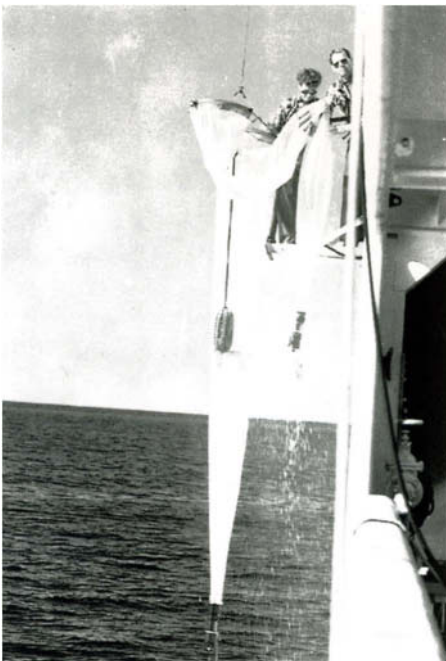
Figure 4.1 A 'Bongo' zooplankton sampler, consisting of duplicate plankton nets, being retrieved on board a research vessel.
