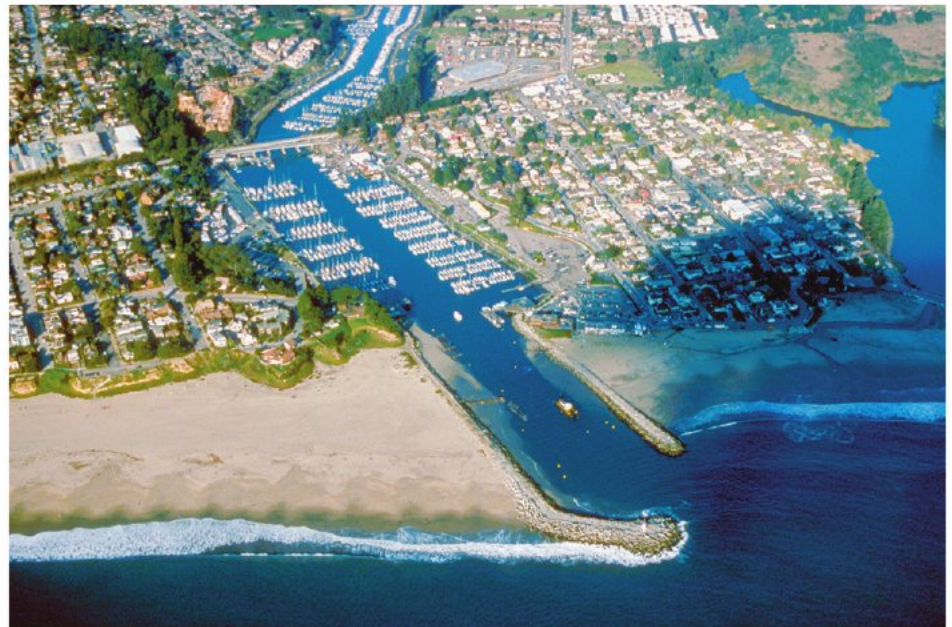
FIGURE 10.21 Jetties at Santa Cruz Harbor, California. These jetties protect the inlet to Santa Cruz Harbor and interrupt the flow of sand, which is toward the right (southward). Notice the buildup of sand to the left (upcoast) of the jetties and the corresponding erosion to the right (downcoast).
