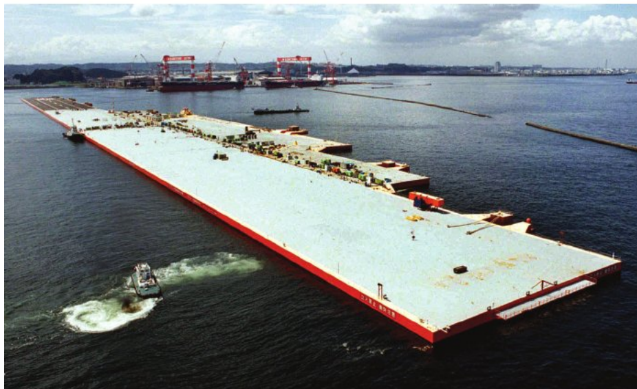
FIGURE 8.6 Floating runway, Japan. This floating runway called “Mega-Float” was built offshore Yokosuka in Tokyo Bay, Japan, and is the world’s largest, with a length of 1000 meters (3300 feet). Stable structures such as runways and bridges can use submerged pontoons to float at the ocean’s surface as long as the majority of the structure’s mass is below wave base.
