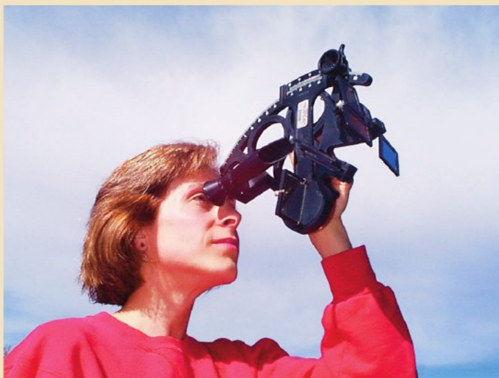
FIGURE 1D Using a handheld sextant. This sextant is similar to the ones used by early navigators to determine latitude.
