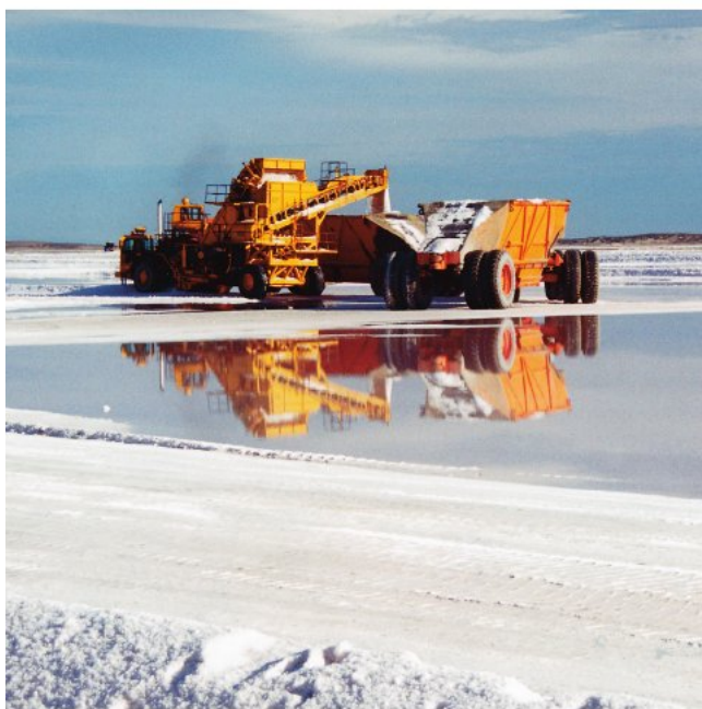
FIGURE 4.26 Mining sea salt. A salt mining operation at Scammon's Lagoon, Baja California, Mexico. Low-lying areas near the lagoon are allowed to flood with seawater, which evaporates in the arid climate and leaves deposits of salt that are then collected.
