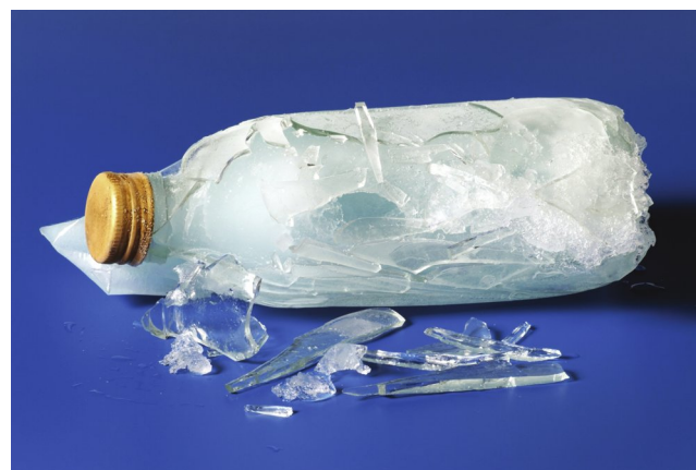
FIGURE 5.14 Glass bottle shattered by frozen water. This glass bottle was filled with water, sealed, and put into a freezer. As water freezes, it expands by 9% as it forms hydrogen bonds and forms an open lattice structure, which increased the pressure and caused the bottle to fracture.
