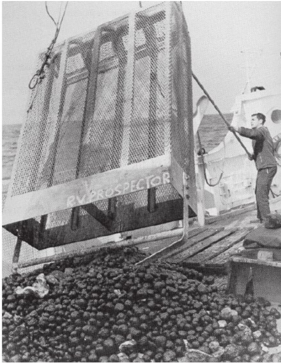
FIGURE 4.27 Mining manganese nodules. Manganese nodules can be collected by dredging the ocean floor. This metal dredge is shown unloading nodules onto the deck of a ship.
