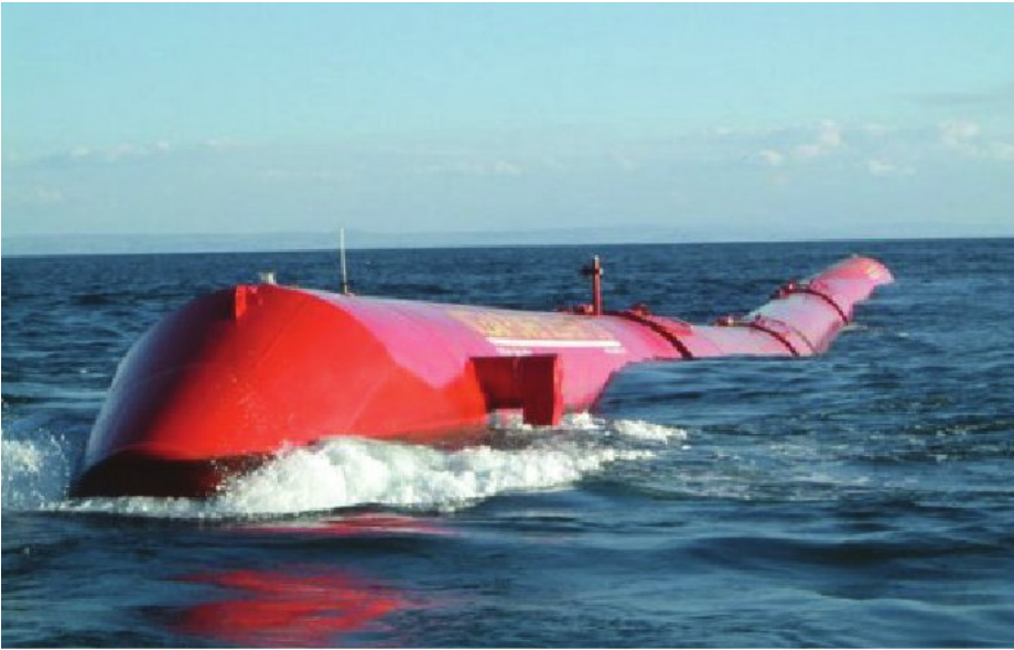
FIGURE 8.28 Harnessing the power of ocean waves. This wave energy device resembles a large segmented floating snake and is designed to flex as waves pass, thus generating electricity. A wave farm of three of these devices is currently generating electricity off northern Portugal, with 25 more planned.
