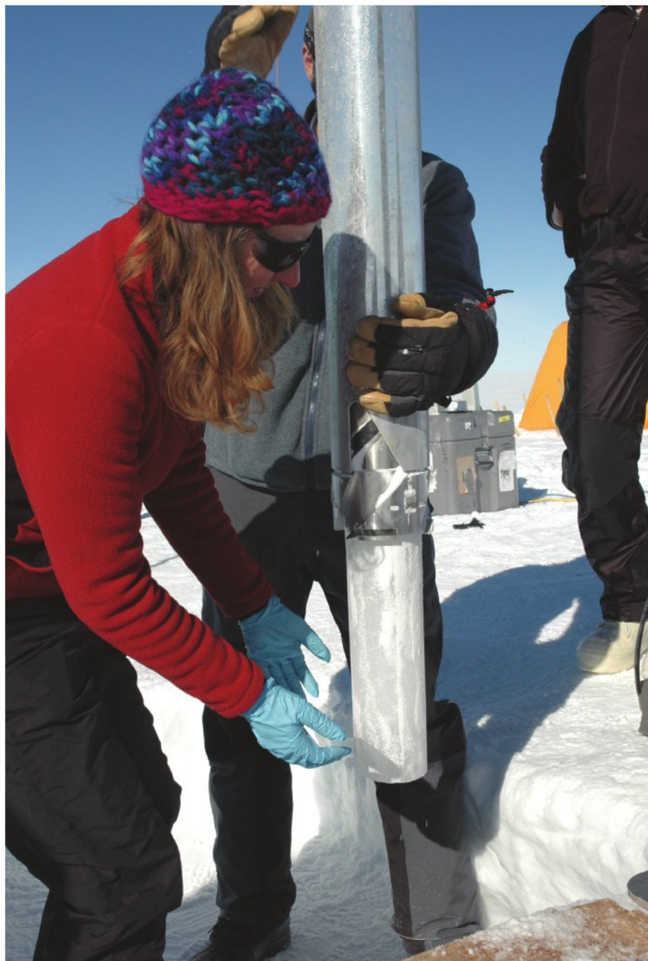
FIGURE 16.2 Researchers extract an ice core from its drilling tube. To reconstruct past temperatures and atmospheric conditions, scientists use natural records of climate change such as this ice core that was recently collected in Antarctica. The annual layers of snow packed in glacial ice preserve a record of climate that stretches back hundreds of thousands of years.
