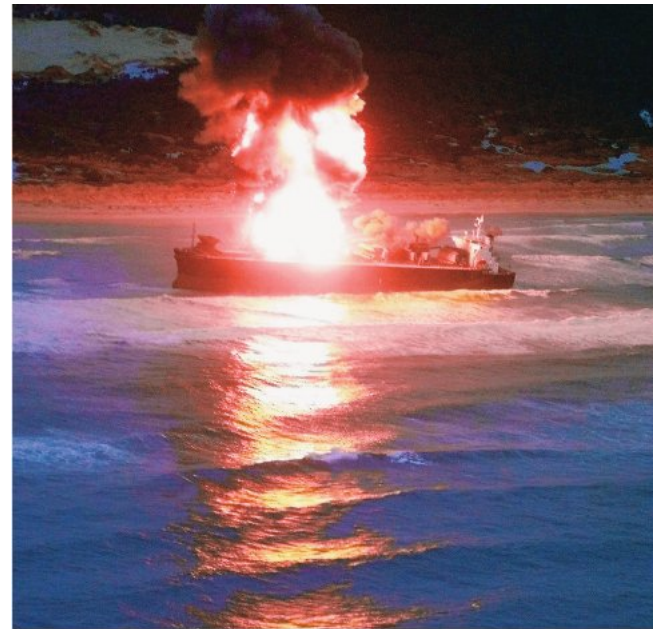
FIGURE 11.21 The New Carissa on fire off the Oregon coast. When the freighter M/V New Carissa ran aground in 1999 in shallow water offshore Coos Bay, Oregon, and began leaking oil, it was intentionally set on fire to prevent further oil from spilling into the ocean.
