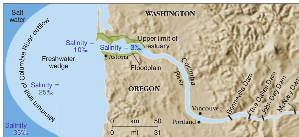
FIGURE 11.8 Columbia River estuary. The long estuary at the mouth of the Columbia River has been severely affected by interference with floodplains that have been diked, by logging activities, and—most significantly—by the construction of hydroelectric dams. The tremendous outflow of the Columbia River creates a large wedge of low-density freshwater that remains traceable far out at sea.
