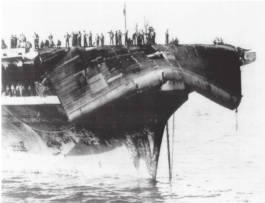
FIGURE 8.13 Wave damage on the aircraft carrier Bennington . The Bennington returns from heavy seas encountered in a typhoon off Okinawa in 1945 with part of its reinforced steel flight deck bent down over its bow. Damage to the flight deck, which is 16.5 meters (54 feet) above still water level, was caused by large waves.
